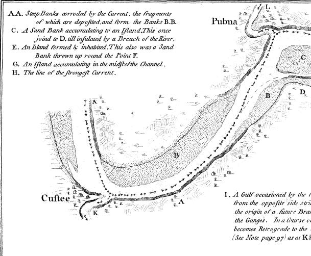
SECTION of a Branch of the GANGES, as a N.B. This is exactly similar to the Section of the winding parts of the
